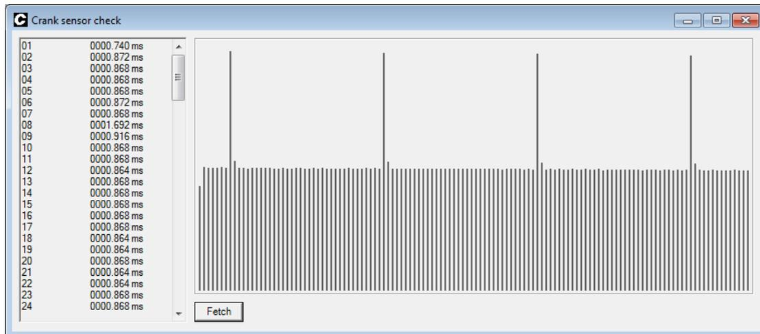
Click '**Diagnostics > Crank sensor check**' and you will see a blank screen. Turn the engine over for few rotations but leave the vehicle ignition turned on. Now click '**Fetch**' to grab the crank sensor data from the ECU itself.
