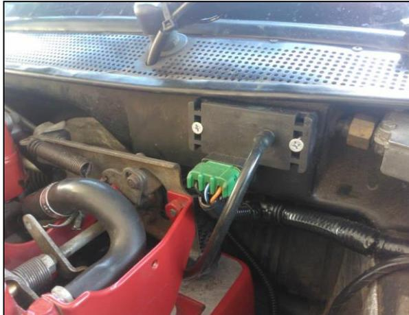
MAP sensor installed in TVR, with vacuum pipe connected to inlet manifold take-off
